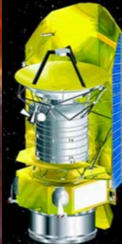
Herschel Space Telescope 2009-2013 3.5m, 55-672 \mu\text{m} (FIR) 3.4 tons 1.5million km from earth, opposite sun
