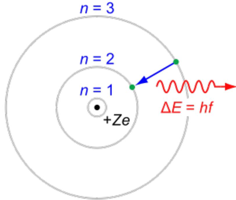
Photon energy  $E$  emitted when electron jumps an orbit
