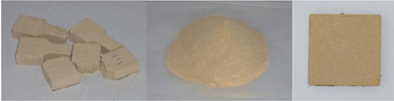
Starch-based thermoplastic wood after forming (left), after grinding (centre) and then after reforming (right). This shows that it can be effectively recycled.
