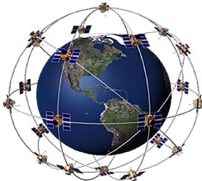
Each satellite **transmits two signals** at 1227 MHz and 1575MHz
