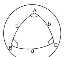
In this figure the angle C is now the azimuth Z of the GP as seen from the AP, which is the angle on a chart relative to North of a line pointing from the AP to the GP. Similarly, the angle a is the declination of the GP as seen from the AP, which is the angle of the celestial body above the Horizon measured by the sextant. Using the spherical trigonometric formulae given earlier we can compute these easily via the formulae
