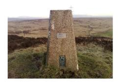
By measuring the angles between the trig points a network of triangles can be constructed linking these points together and hence produce the basis of a map. The triangulation must then be checked periodically by measuring further base lines to high accuracy. From this network of large triangles, smaller triangles can be then constructed and a map built up
