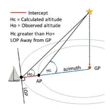
To fix the position of the ship this procedure is repeated for one or more celestial bodies, and the ship then lies on the intersection of the various calculated position lines. See [??] for more details of this method.
