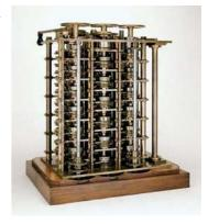
aided by Ada Lovelace) to produce in 1832 a small working model of the calculating section of Difference Engine No. 1, which operated on 6-digit numbers and second-order differences. Unfortunately, the full project was not accomplished successfully, and it was abandoned in 1842.
