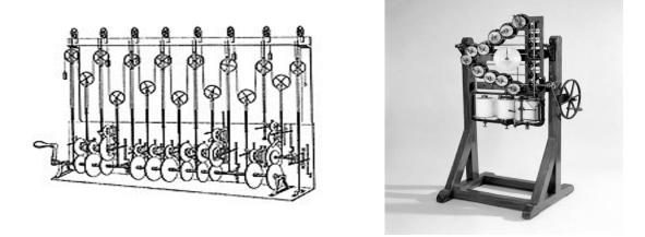
The Kelvin tidal computer is an example of what we now would call and 'analogue computer'. Once set up with data from previous tidal events, it could calculate with great accuracy the height of future tides. It was so good that it was used for the tidal calculations for the D-day landings, and similar computers were used until the 1960's. At this point they were replaced by the modern electronic computer which we will discuss next.
