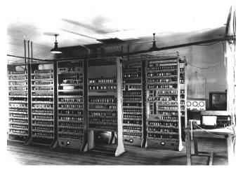
EDSAC was subsequently used to do many scientific computations in both pure and applied mathematics. Although EDSAC was modest in terms of modern-day computers (there were only 18 operation codes, just 1024 words of memory, later extended to 1024 and instructions were executed at a rate of approximately 650 per second.) it was far faster than any other machine in use in Cambridge at the time, and transformed work there,
