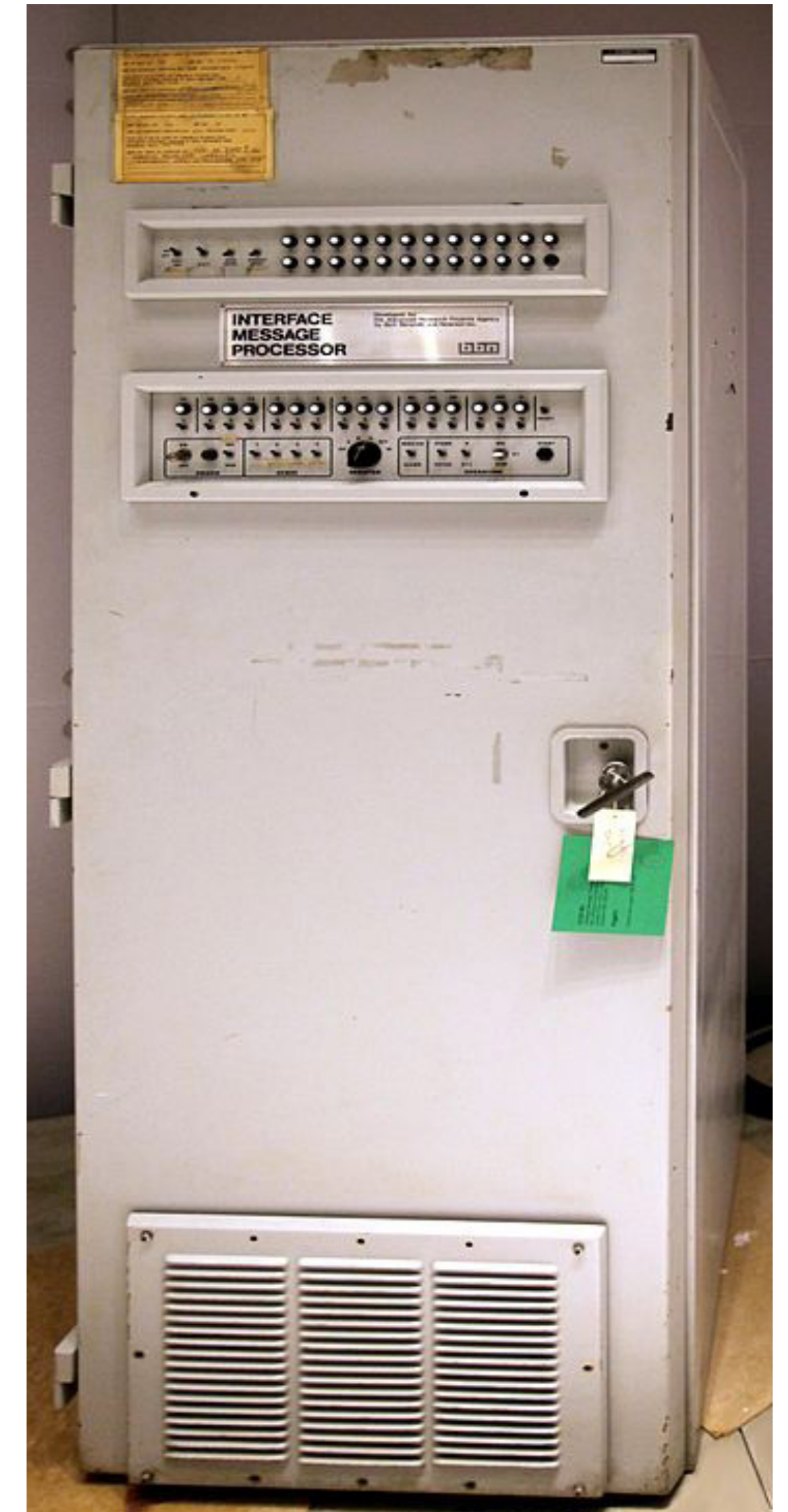
One of the many essential steps in the creation of what would become known as the internet occurred in 1968 when ARPA contracted BBN Technologies to build the first routers, known as Interface Message Processors or IMPs, which enabled ARPANET to become operational the following year. (Photo courtesy of Steve Jurvetson under a CC BY 2.0 license)
