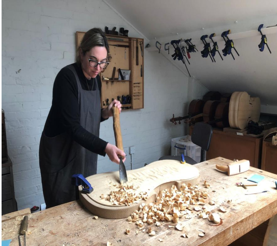
Making the prototype “Open String” cello
